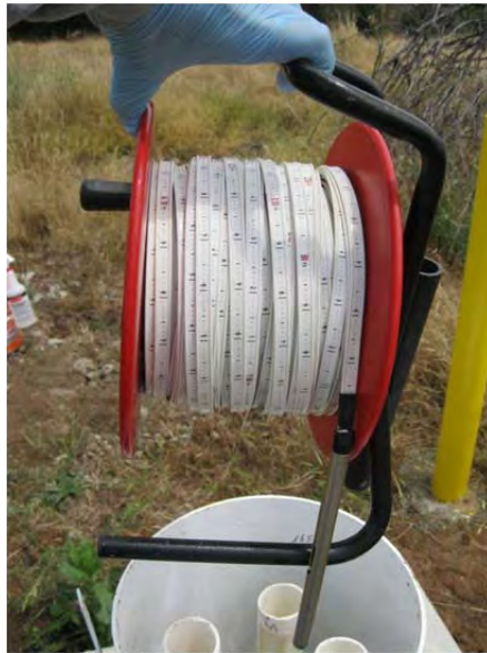
FIGURE 4-3. WELL SOUNDING PROBE AND TAPE
